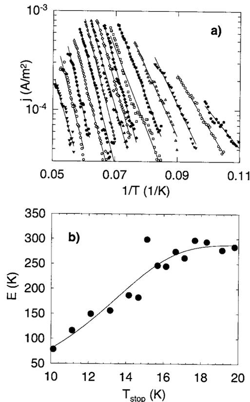
FIG. 9. (a) The TSD current spectra of o-TaS<sub>3</sub> obtained on sample III for partial depolarization with  $T_{\text{pol}}=30$  K,  $h=10$  K/min, and  $E_{\text{pol}}=45$  V/cm. (b)  $E_{\text{eff}}$  as a function of  $T_{\text{stop}}$  in partial polarization extracted from the TSD spectra in Fig. 9(a).
