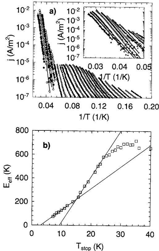
FIG. 6. (a) This TSD current spectra of  $K_{0.3}MoO_3$  obtained for partial depolarization with  $T_{pol}=50$  K,  $E_{pol}=1.4$  V/cm, and  $h=7$  K/min. (b)  $E_{eff}$  as the function of  $T_{stop}$  in partial polarization as extracted from the TSD current spectra of  $K_{0.3}MoO_3$  in Fig. 6(a).
