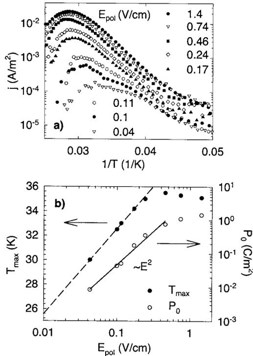
FIG. 4. (a) The TSD current spectra of  $K_{0.3}MoO_3$  obtained for various  $E_{pol}$  with  $T_{pol}=50$  K and  $h=7$  K/min. (b)  $P_0$  and  $T_{max}$  as the function of  $E_{pol}$  extracted from the TSD current spectra in Fig. 4(a). The full line indicates the quadratic  $E_{pol}$  dependence and the dashed line provides the extrapolation of  $T_{max}$  to low poling fields.
