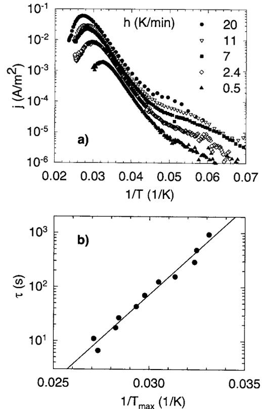
FIG. 5. (a) The TSD current spectra of  $K_{0.3}MoO_3$  obtained for various  $h$  with  $T_{pol}=50$  K and  $E_{pol}=1.4$  V/cm. (b)  $\tau_{eff}$  as the function of  $T_{max}$  for different  $h$  as extracted from the TSD current spectra of  $K_{0.3}MoO_3$  in Fig. 5(a). The line indicates activated  $T_{max}$  dependence with  $E_{act}=700$  K and  $\tau_0=10^{-8}$  s.
