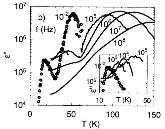
FIG. 3. Effective  $\epsilon''(T)$  calculated from the TSD spectra in Fig. 2 compared to the directly measured (Refs. 3 and 4)  $\epsilon''(T)$  for (a)  $K_{0.3}MoO_3$  and (b)  $o-TaS_3$  at several frequencies between  $10^8$  and  $10^2$  Hz. For TSD the effective frequency is calculated as  $1/(2\pi\tau_{eff})$  with  $\tau_{eff}$  for  $\alpha$  from Table I. For  $o-TaS_3$  the  $\alpha$  process is presented in the main panel and the  $\beta$  process in the inset for clarity.
