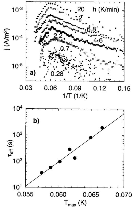
FIG. 8. (a) The TSD current spectra of o-TaS<sub>3</sub> obtained on sample III for various  $h$  with  $T_{\text{pol}}=30$  K and  $E_{\text{pol}}=45$  V/cm. (b)  $\tau_{\text{eff}}$  as the function of  $T_{\text{max}}$  for different  $h$  extracted from the TSD spectra in Fig. 8(a). The line indicates the activated  $T_{\text{max}}$  dependence with  $E_{\text{act}}=420$  K and  $\tau_0=7 \times 10^{-10}$  s.
